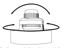
Move the camera vertically up and down or rotate the camera to change the camera lens angle.
